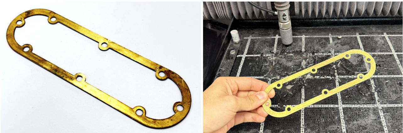
Fig.48: Brass gasket result
