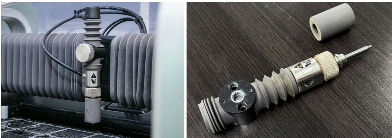
Fig.10: Water jet nozzle
