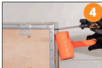
Use a hammer to knock the top panels off from the metal tabs
