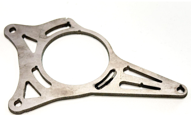
Fig.41: MTB chainring bracket result
